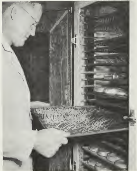
Checking germination of seeds on moist paper in a temperature-controlled chamber, during a germination test.
